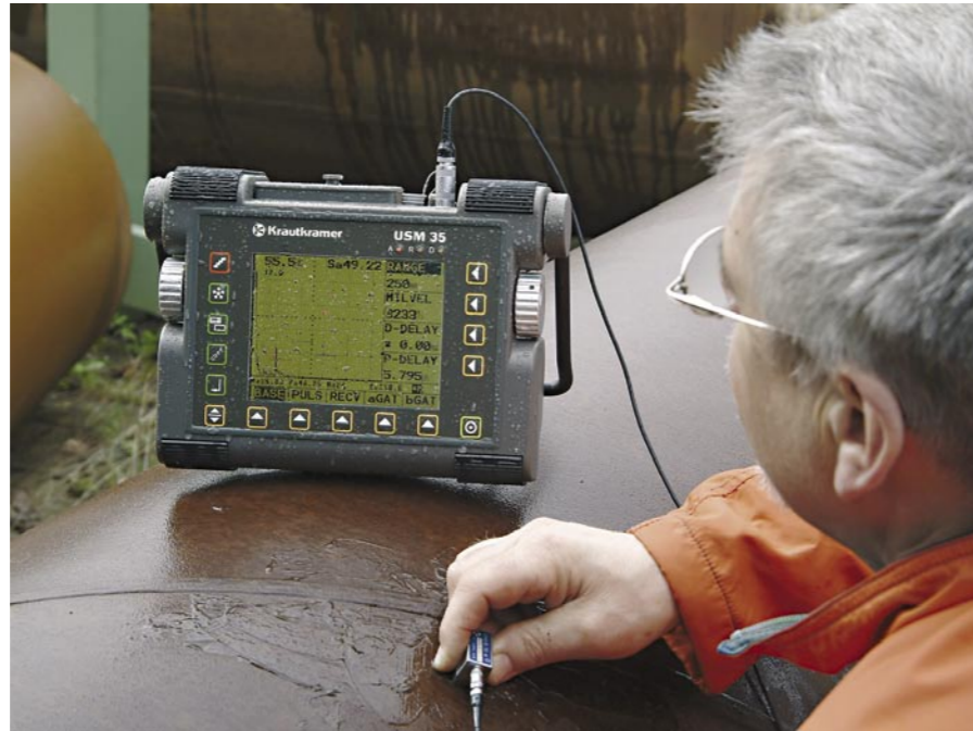
Inspection of a weld
