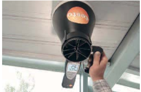
testo 417, e.g. for monitoring the air input at a plate ventilation outlet
