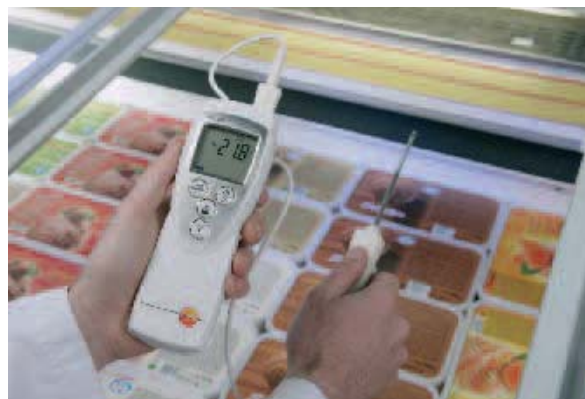
Air temperature measurement in refrigerated display counters and freezers
