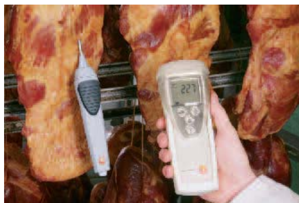
Measurement of penetration temperature when smoking foods, wireless radio transmission of measurement data
