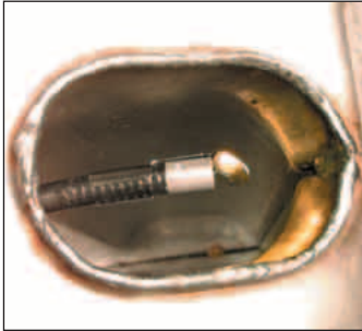
Fast and complete heat exchanger inspection with mirror accessory
